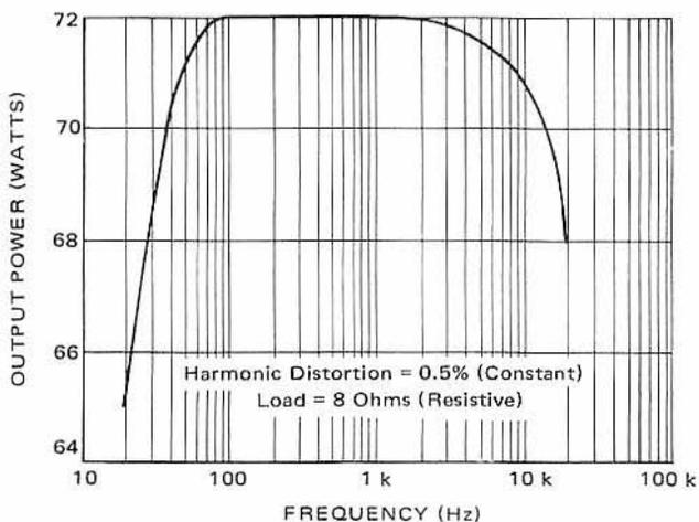
Figure 5-43 — 50-W-Amplifier Output Power versus Frequency
