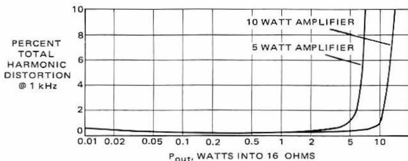
Figure 5-25 – Harmonic Distortion versus Power Output
