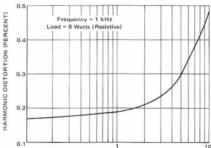
Figure 5-33 — Harmonic Distortion versus Output Power
