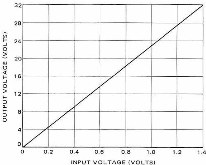
Figure 5-15 — DC Servo Amplifier Gain Characteristics
