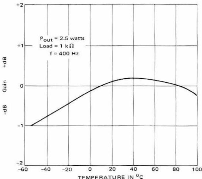
Figure 5-11 — Voltage Gain as a Function of Temperature
