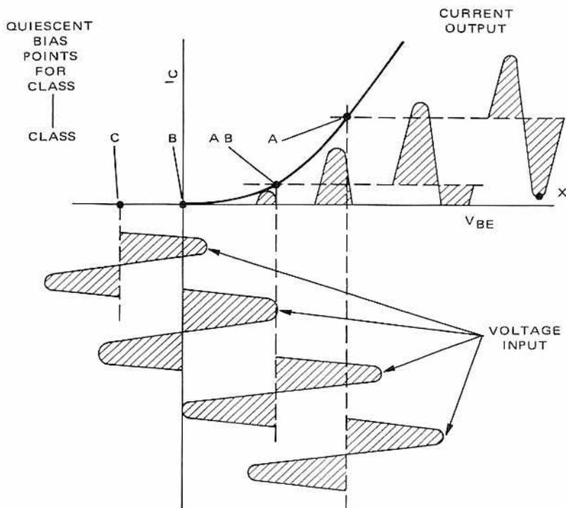
Figure 5-1 — Waveshapes of Classes of Operation
