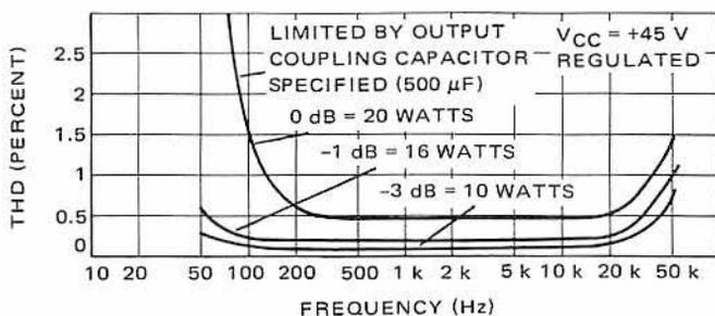
Figure 5-35 — Distortion versus Frequency Response
