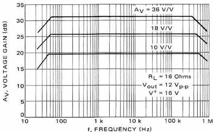
Figure 5-19 – Frequency Response of IC Audio Amplifier
