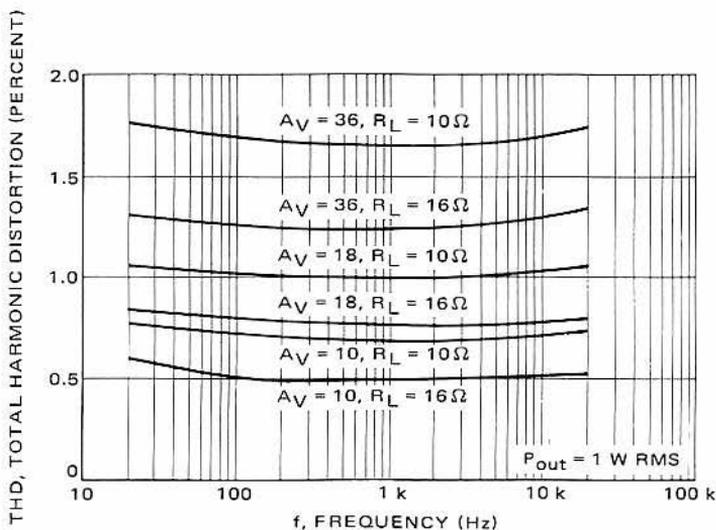
Figure 5-20 – Total Harmonic Distortion of IC Audio Amplifier
