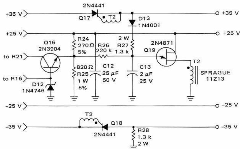
Figure 5-42 — 50 W Amplifier Delayed Switching Circuit
