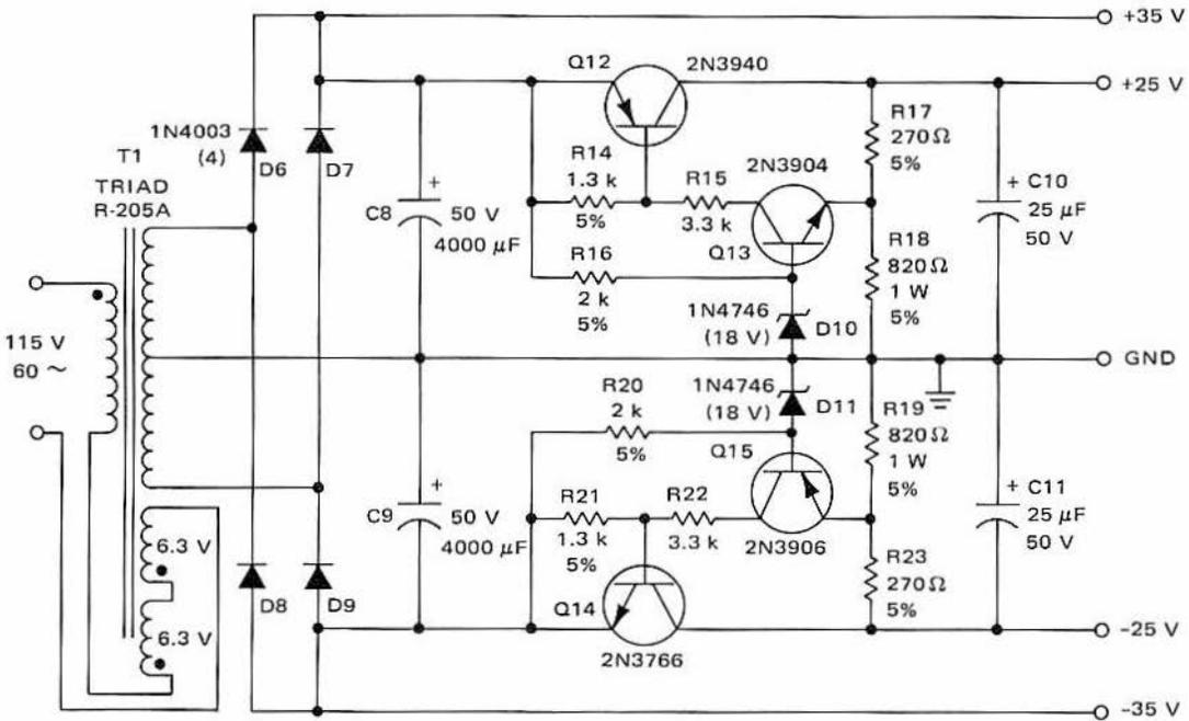
Figure 5-41 — 50 Watt Amplifier Power Supply
