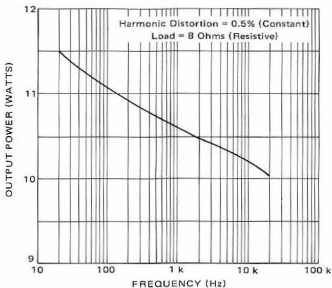
Figure 5-29 – Output Power versus Frequency
