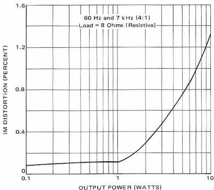
Figure 5-31 – Intermodulation Distortion
