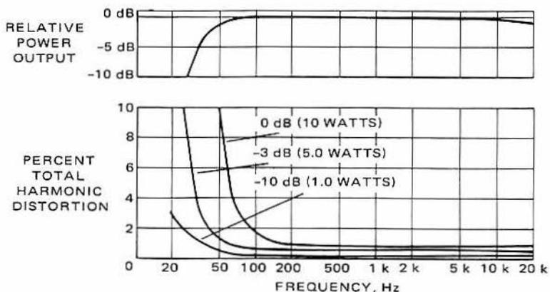
Figure 5-27 – 10 W Amplifier Bandwidth and Distortion Characteristics
