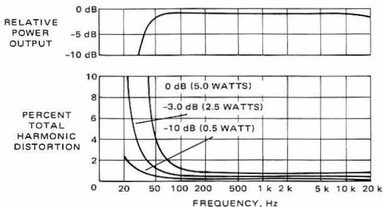
Figure 5-26 – 5 W-Amplifier Bandwidth and Distortion Characteristics
