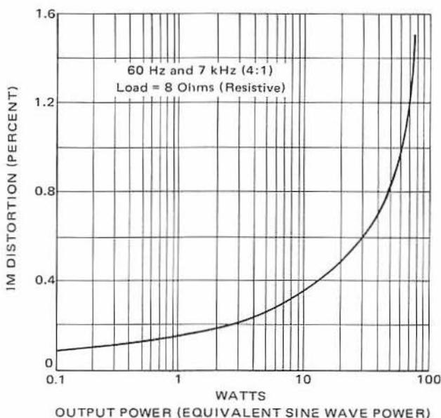
Figure 5-45 — 50-Watt-Amplifier Intermodulation Distortion
